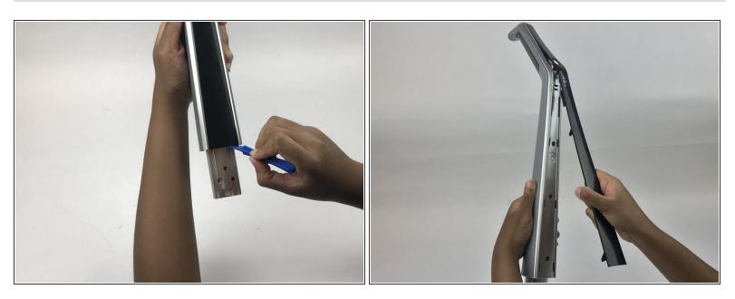
• Use a plastic opening tool to carefully pry the black cover off of the handle.
