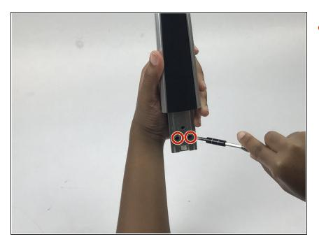
Remove two 15mm Phillips #1 screws from the handle.
