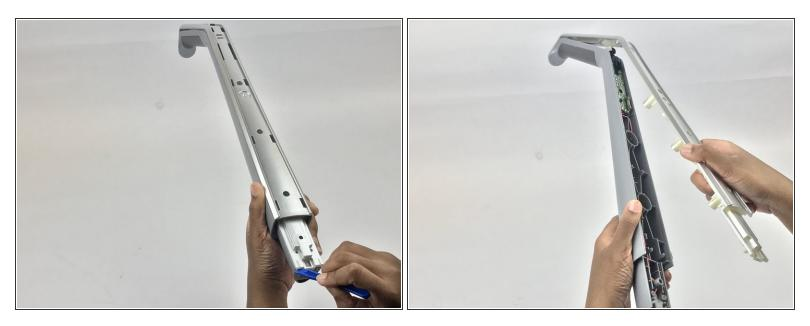
• Remove the silver plastic cover using the plastic opening tool.
