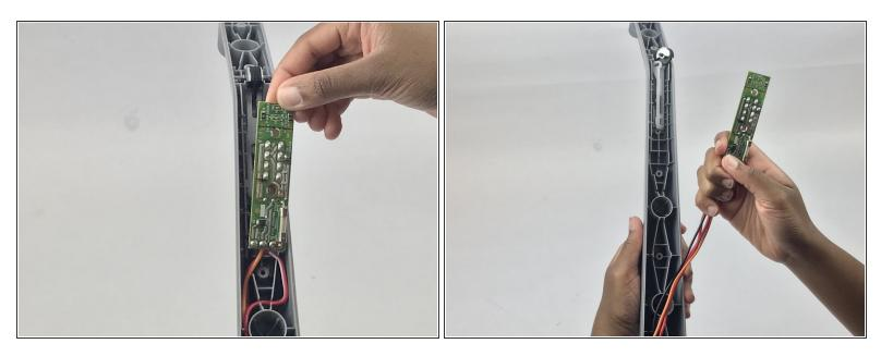
• Carefully pull the motherboard out with its attached wires.
