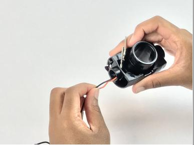
Remove the angled neck and feed the prongs out through their channels.
