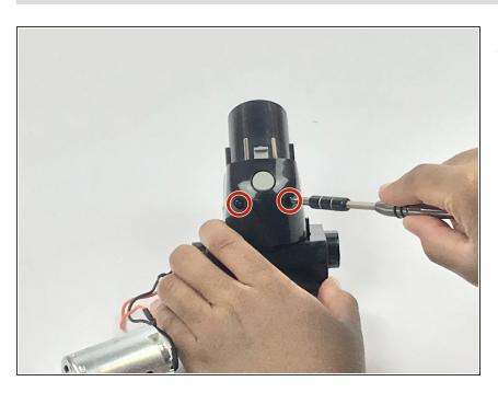
Remove the two 7.5mm Phillips #1 screws from the main body.
