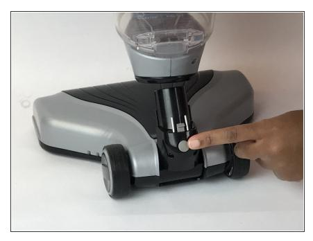
Detach the rolling assembly from the body by pushing the button found at the base.
