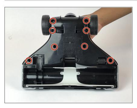
Remove the eight 4mm Phillips #1 screws from the bottom panel.
