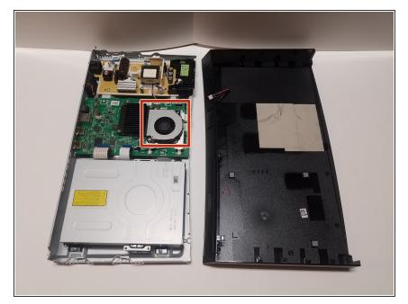
Fan A is located on top of the motherboard and is screwed into a stand by two 6.5mm screws. The stand is also connected to the motherboard.
