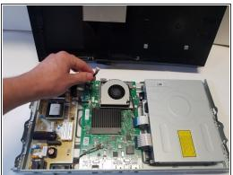
There is one group of wires located towards the front of the case and attached directly to the motherboard and the case. Using two fingers in a pinching motion, release the wire from the clip and disconnect it.
