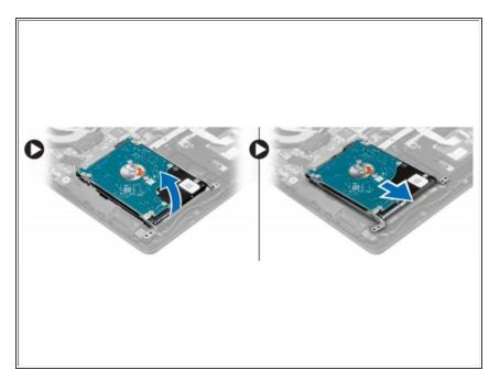
Lift the hard drive assembly in an upward direction to release it from its compartment on the computer. Remove the hard drive from the computer.
