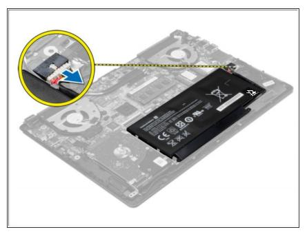
• Disconnect the battery cable from its connector on the system board.
