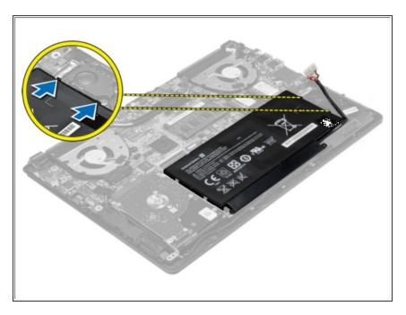
• Release the tabs that secure the battery in the battery bay.
