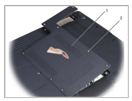
• Turn the computer upside-down, loosen the eight captive screws on the cover and remove the cover.
