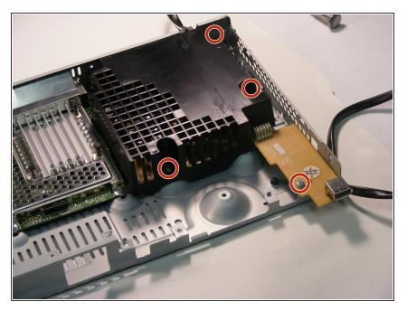
Unscrew the 1.2mm screws labeled with a red circle and remove the power supply from the player.
