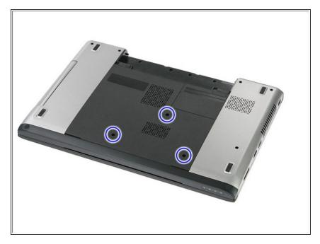
Remove the screws that secure the access panel to the base of the computer.
