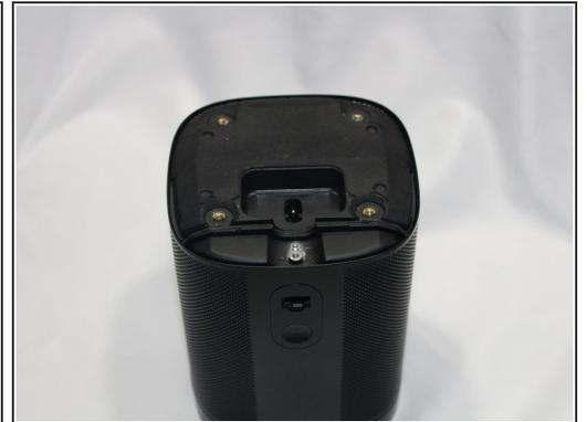
**i** The protective cover clip is very thin and deforms easily.
