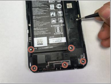
Remove the twelve 2.5mm Phillips #0 screws from the back of the phone.
