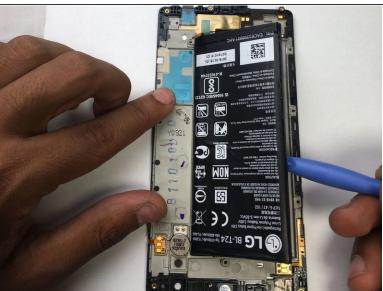
Use a spudger and plastic opening tool to carefully pry up the battery.
