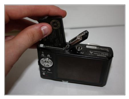
Remove the battery and the SD card.
