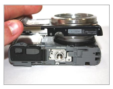
Separate the front of the camera from the main body carefully.
