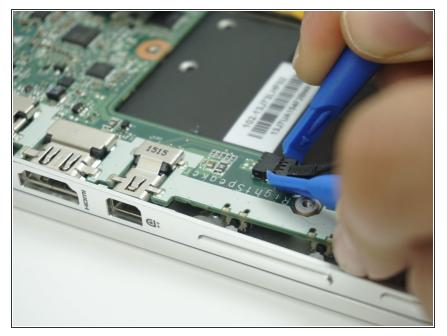
Using two plastic opening tools, Disconnect the right speaker cable from the motherboard.
