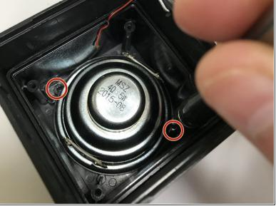
Remove the speaker's two 10 mm screws that are located in its base then take the driver out of the speaker.
