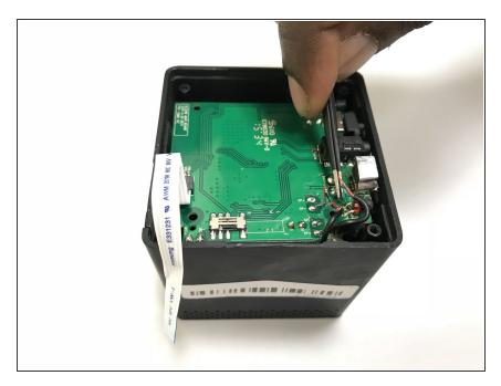
Remove the red/black wires in addition to the blue/white wires using the tweezers.
