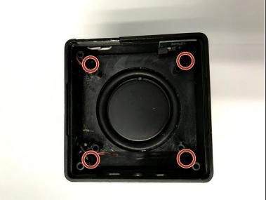
Remove the speaker's four 10 mm base screws.
