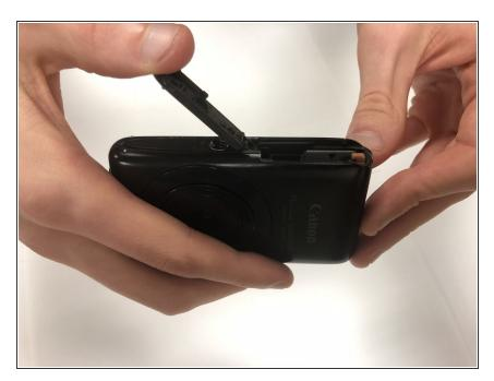
Once the hatch is slid so the end is overhanging the edge of the camera, you will be able to lift it open.
