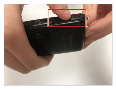
The hatch covering the memory card will slide open towards the corner of the device.
