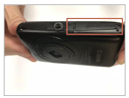
The battery compartment is located on the bottom of the camera, below the user interface panel.
