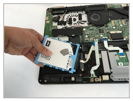
• Lift the hard drive up and out of the laptop.
