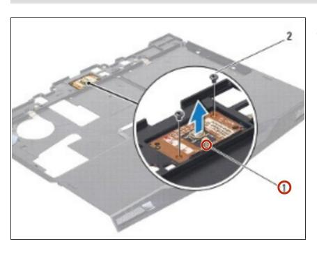
Lift the power button board off the palm rest assembly.
