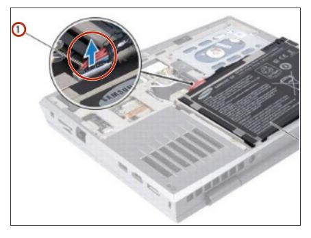
Route the battery pack cable in the routing guide
