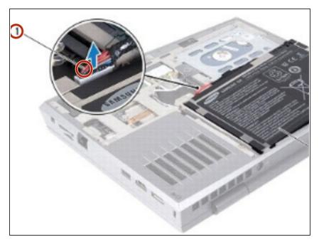
Disconnect the battery pack cable from the connector on the system board.
