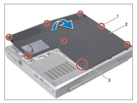
Tighten the eight screws that secure the base cover to the computer base.
