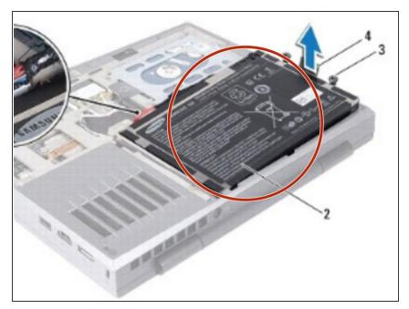
Place the **NEW** battery pack in the battery bay and replace the two screws that secure the battery pack to the computer base.
