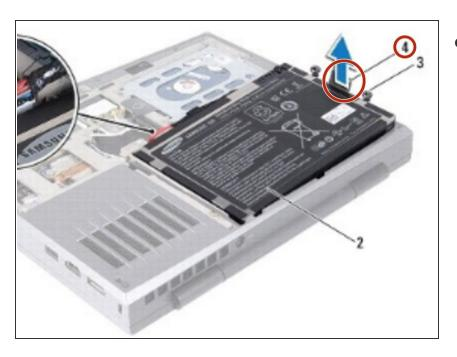
Using the pull-tab, lift the battery pack off the computer base.
