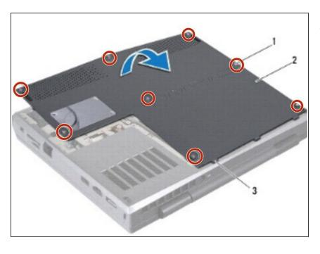
Loosen the eight captive screws that secure the base cover to the computer base.
