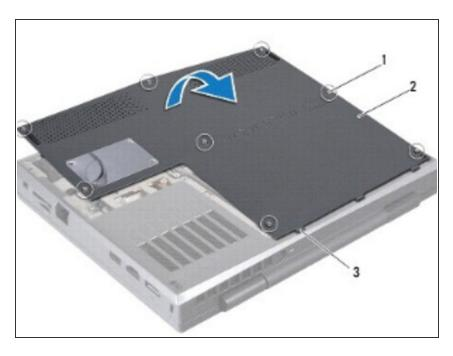
Align the tabs on the NEW base cover with the slots on the computer base and place the base cover in position.
