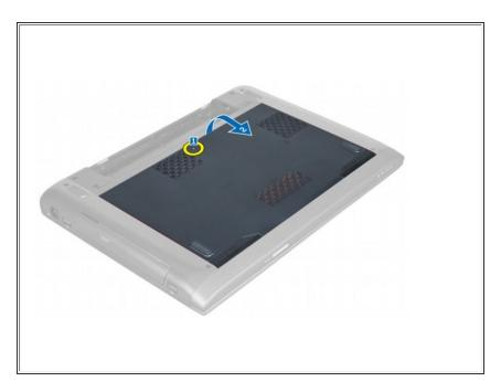
Remove the screw(s) that secures the cover to the computer. Lift the cover upwards.
