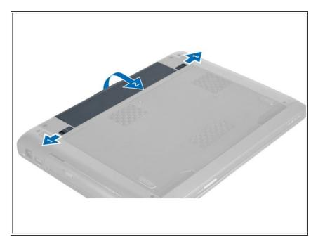
Slide the battery latches to release the battery.
