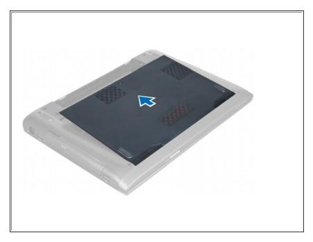
Slide the cover outwards to release it from the notches on the computer.
