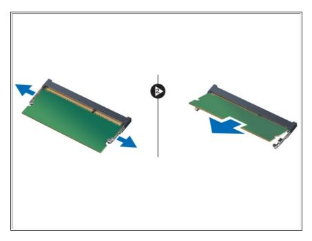
Pry the retention clips away from the memory module until it pops-up. Lift and remove the memory module from its connector.
