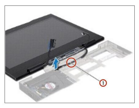
Gently slide the Mini-Card antenna cables out through the slot on the computer base.
