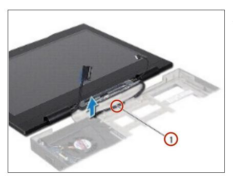
Slide the antenna cables in through the slot on the computer base.
