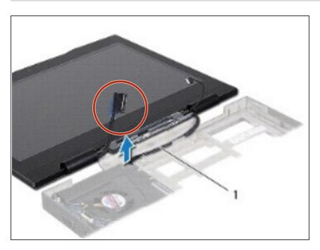
Lift the display assembly off the computer.
