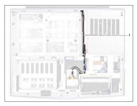
Turn the computer over and route the Mini-Card antenna cables through the routing guides on the computer base.
