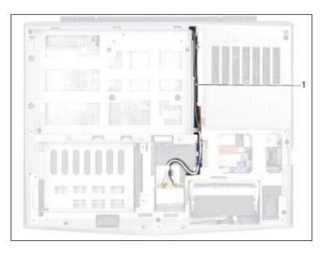
The routing of the Mini-Card antenna cables and remove them from the routing guides on the computer base.
