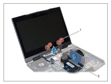
Place the **NEW** display assembly in position and replace the four screws that secure the display assembly to the computer base.
