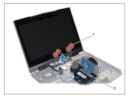
Remove the four screws that secure the display assembly to the computer base.
