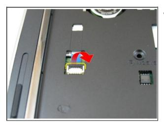
Release the latch on the system board connector and then disconnect the power button cable.
