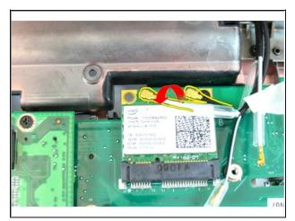
Disconnect the wireless local area network (WLAN) antenna cable.
