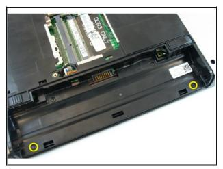
Remove the screws that secure the hinge cover.
