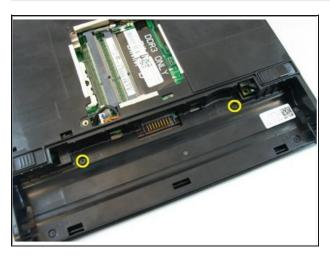
Remove the screws in the battery compartment.
