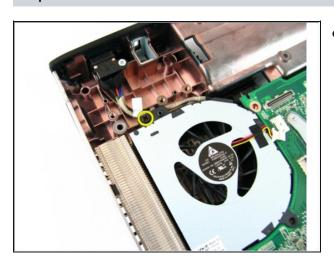
Remove the screw that secures the system fan.
