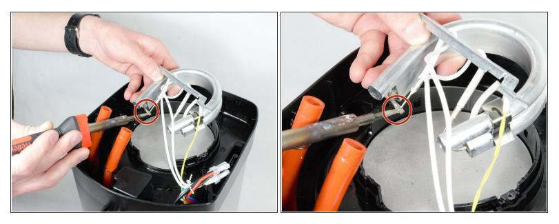
If heating contacts are connected, use a soldering iron to <u>desolder</u> the bond between metal contact points.
