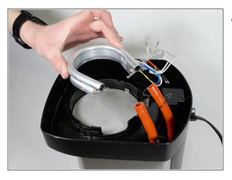
• Remove and replace the defective heating element.
