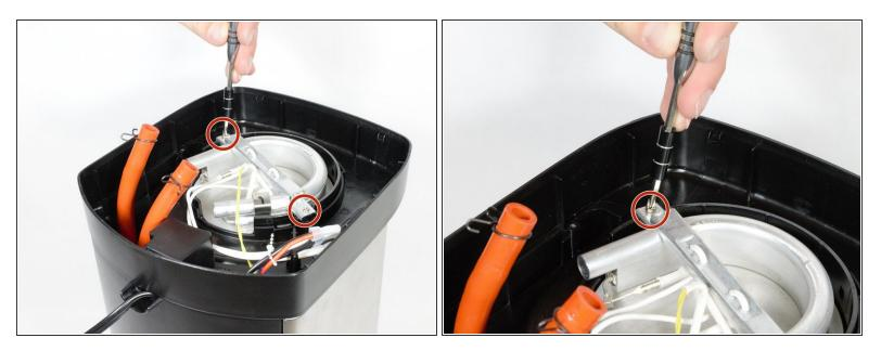
Use the bit driver with the extension attachment with the PH1 Phillips bit to remove the two 18mm long screws on heating element plate.
