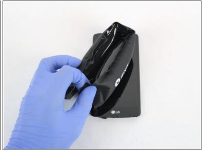
Heat the screen up using a heat gun (or the IOpener) to loosen up the screen. The heat gun needs to be moved around the edges of the phone in order to equally heat the edges.
