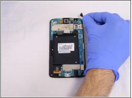
The front camera can be removed in a similar way as the rear camera. See previous step.
