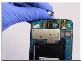
Remove the speaker using the Spudger.
