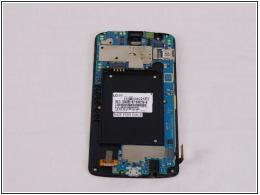
Remove the screen connector using the Spudger.
