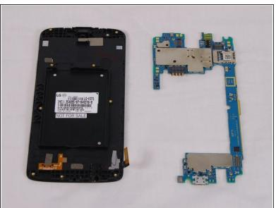
Using a Spudger, separate the motherboard from the back frame.
