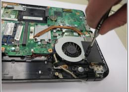
Remove the two 5mm screws on the fan assembly using a Phillips #0 screwdriver.
