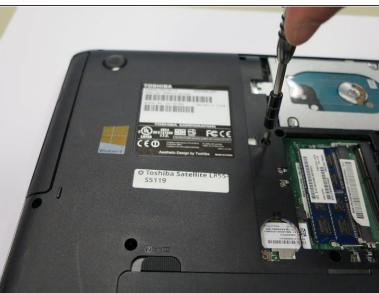
Using a Phillips #0 screwdriver, remove the single 3mm screw.
