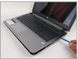
Using a plastic opening tool, begin to pry edge of case away from the laptop. Work around the edges until all sides, except back, are open.
