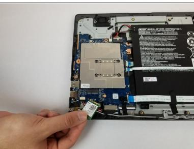
Slide out the Wifi card from its slot by pulling parallel to the board.
