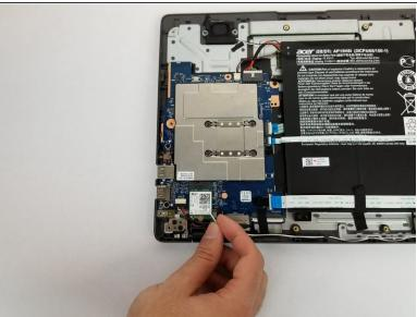
Disconnect the two antenna cables from the Wi-Fi card.
