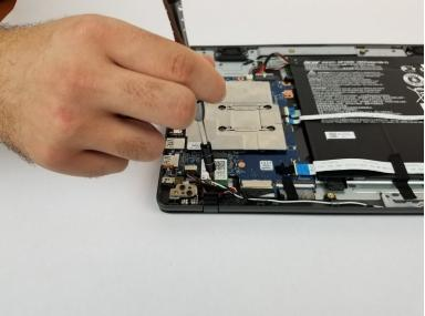
Remove the single 5mm Phillips #0 screw from the Wi-Fi card.
