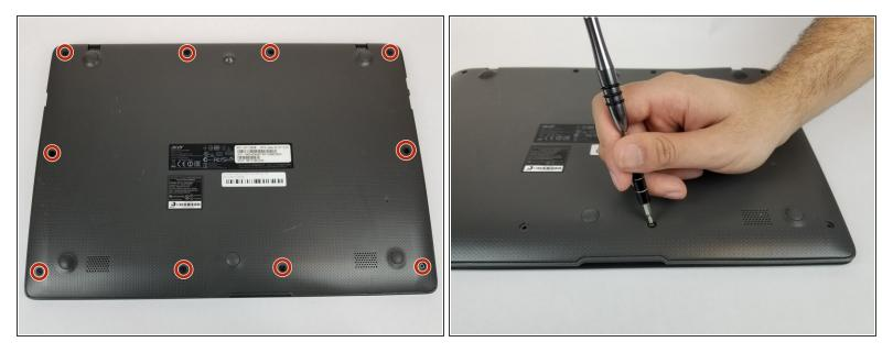
• Remove the ten 7mm Phillips #0 screws from the bottom.
