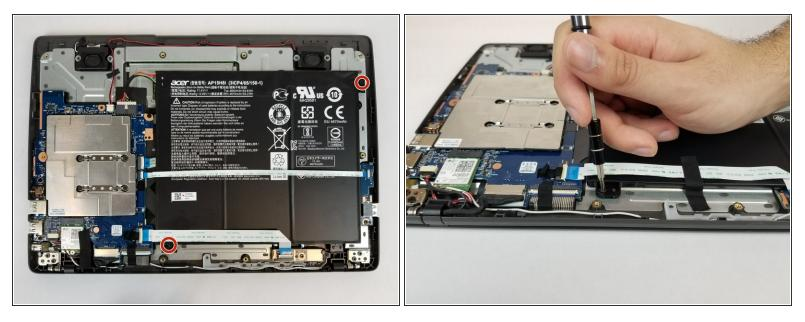
• Remove the two 5mm Phillips #0 screws from the battery.
