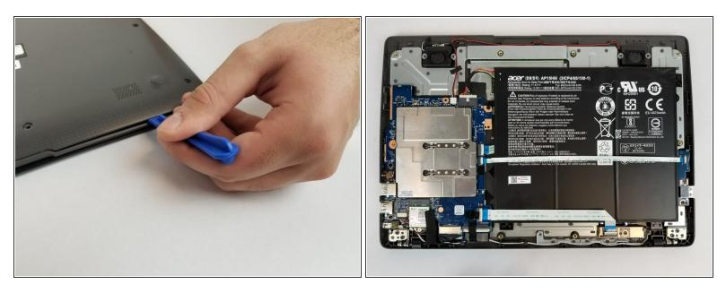
Insert a plastic opening tool under the bottom cover and slid it around the perimeter until all of the clips release.
