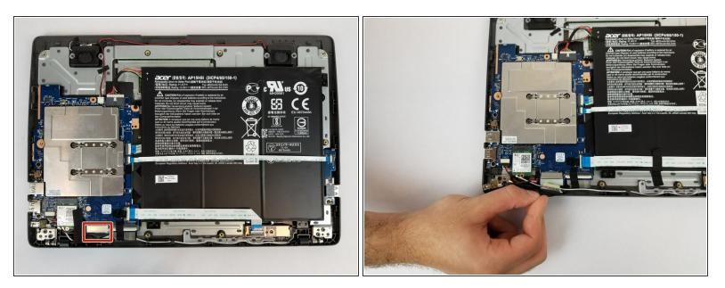
Disconnect the display cable by pulling it down and towards you.
