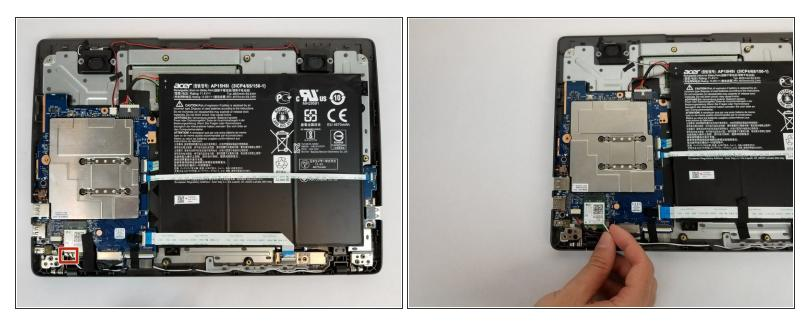
Disconnect the two antenna cables from the Wi-fi card.
