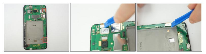
Use the Plastic Opening tools to gently dislodge the two connection on the top and bottom right of the phone from the inside of the phone.
