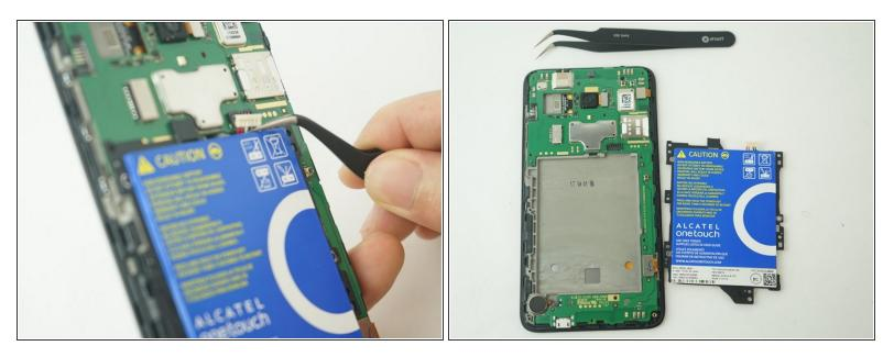
Use a pair of tweezers to pull the battery connector from its port.
