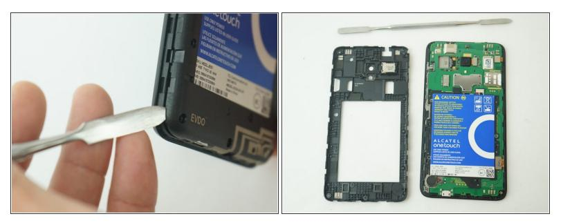
• Gently pry off the Mid frame from the phone using a Metal Spudger.
