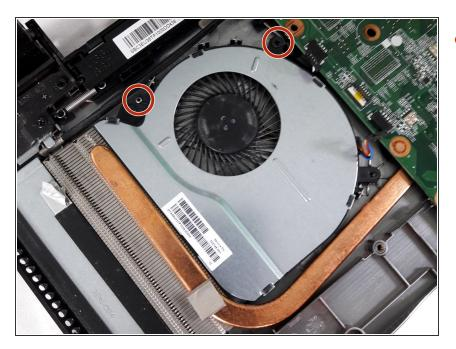
Remove the three x 5.5 mm restraining screws.
