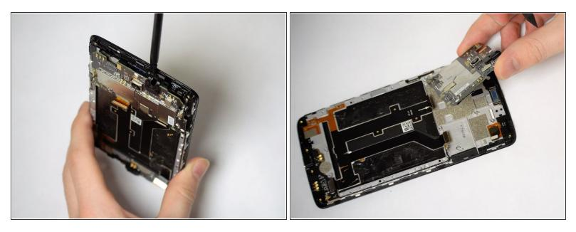
• Gently pry off the large circuit board using the plastic spudger.
