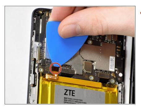
On the top left of the battery, flip the metal clips with a pick and remove the battery ribbon from the shell.
