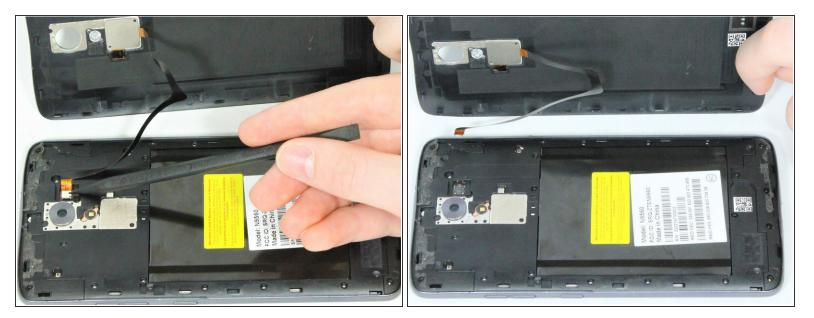
After removal of the two 3.4mm JIS 00 screws, disconnect the connector that attaches the ribbon wire from the main part of the phone.
