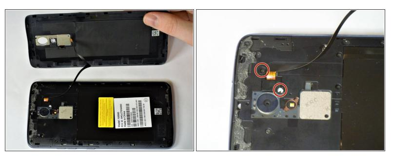
(i) Carefully undo the ribbon wire for the fingerprint scanner before full removal of the backing.
