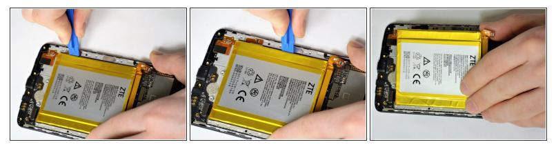
• Using the iFixit opening tools carefully pry the edges of the battery away from the casing.
