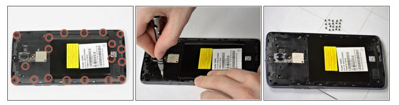
Remove the nineteen 3.4mm JIS 00 screws on the perimeter of the back using the JIS 00 screwdriver.
