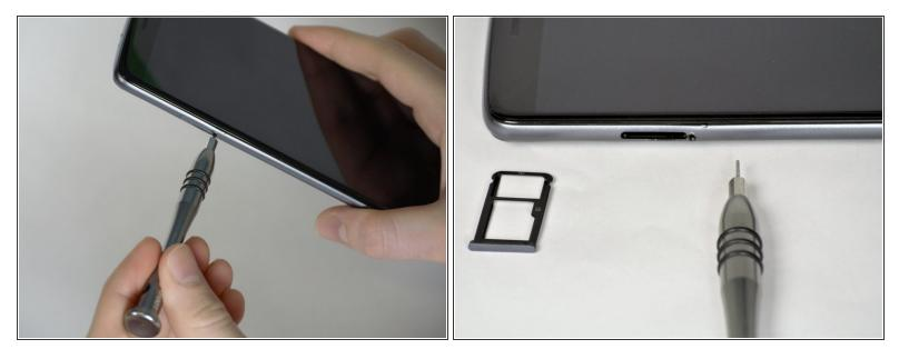
Before any disassembly, make sure the phone is powered off.
