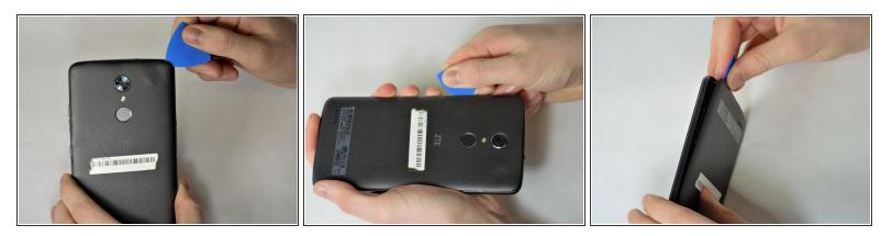
• Starting at one corner, wedge the plastic opening pick underneath the plastic backing to start undoing the tabs that connect the backing to the phone. There are 3 tabs on top and bottom, and 6 on each side.
