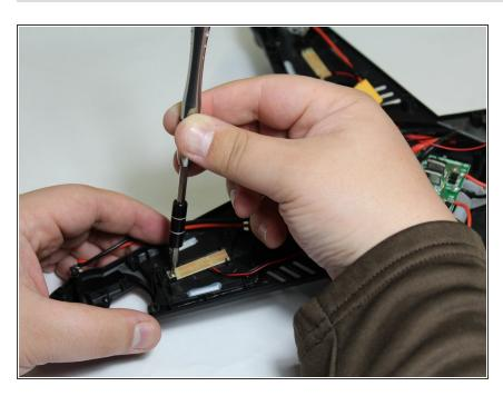
Remove 6mm Phillips #0 screw from the LED strip.
