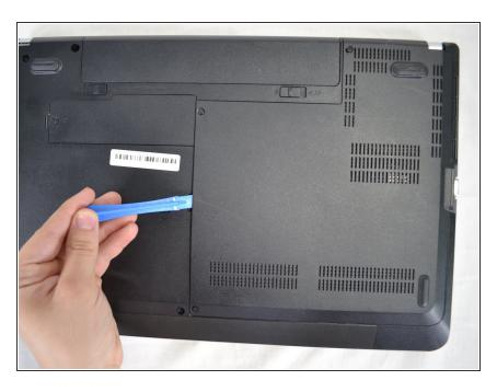
• Use a plastic opening tool to pry off the bottom panel.
