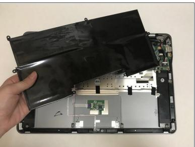
Use the plastic opening tool or your fingers to pry the battery up and pull it from the laptop.
