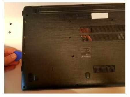
Run a pick between the bottom cover and the device around the edge of the laptop and unclip the cover from the rest of the device.
