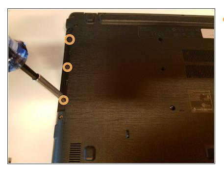
Unscrew the three 2.5 mm Phillips head screws underneath the optical drive bay.
