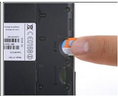
• Push to eject and remove the MicroSD and SIM cards (if installed).
