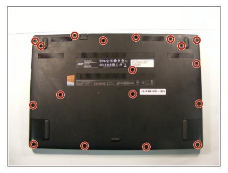
Remove the 18 marked screws
