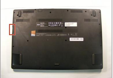
Use the spudger to slowly work your way around the perimeter starting at the marked location to pop the bottom cover off.
