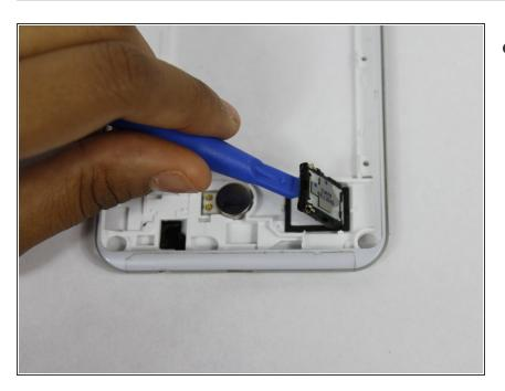
• Using a plastic opening tool, pry the rear facing speaker from the panel.
