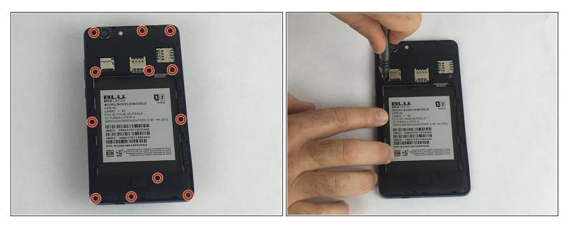
• Remove twelve 3mm Phillips #000 screws from the rear plate.
