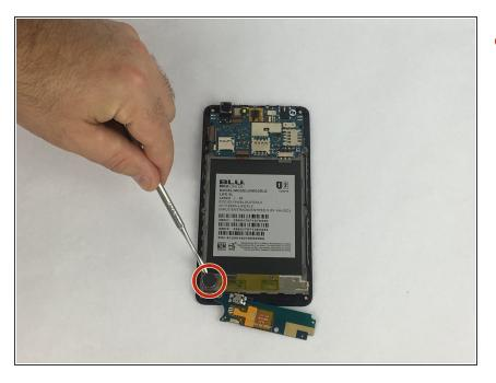
Remove the haptic motor at bottom left of the device. This will require a prying tool, as the motor is glued to the device.
