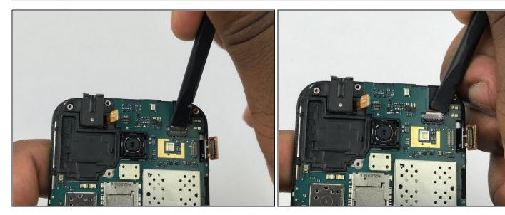
• Use the flat end a spudger to disconnect the front-facing camera cable connecter.
