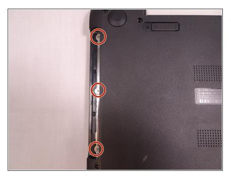
Remove the three 2mm Phillips #00 screws found underneath the disk drive.
