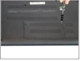
Remove the two Phillips #1 screws from the RAM panel.
