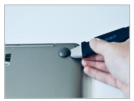
Remove the two round rubber feet at the hinge-edge of the laptop.
