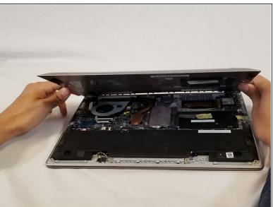
Using a plastic opening tool pry the back panel off of the laptop.
