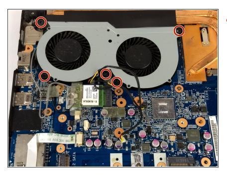
Use a #0 Phillips head screwdriver and unscrew the five 7mm screws holding the fan in place.
