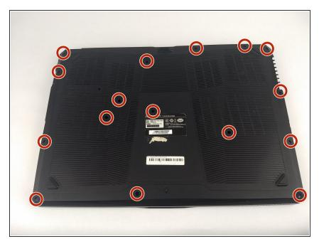
Use a #0 Phillips head screwdriver and unscrew the sixteen 7mm screws on the back of the device.
