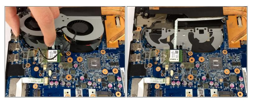
Lift the Graphics card fan out and replace with the replacement fan.
