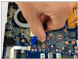
To take out the Graphics card fan it is necessary to disconnect the two Graphic card fan cables.
