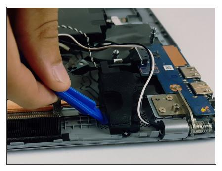
Using the plastic opening tool, pry up the right speaker and take it out.
