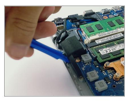
Using the plastic opening tool, pry up the left speaker and take it out.
