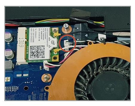
Pull up on the wires circled to disconnect the right speaker.
