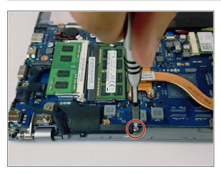
Unscrew the 3.4mm long screw holding the left speaker in place.
