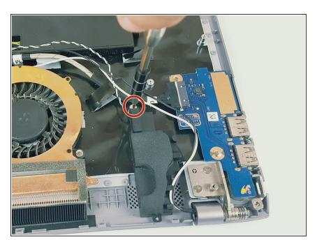
Unscrew the 3.4mm long screw holding the right speaker in place.
