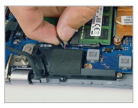
Pull up on the wires to disconnect the left speaker.
