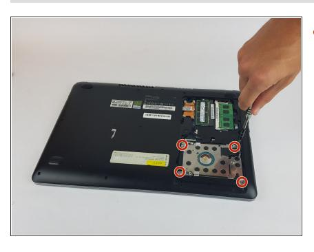
With the cover removed, unscrew all four of the 4.75mm long screws using the Phillips #0 screwdriver.
