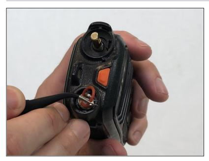
Remove the orange o-ring around volume knob using tweezers.
