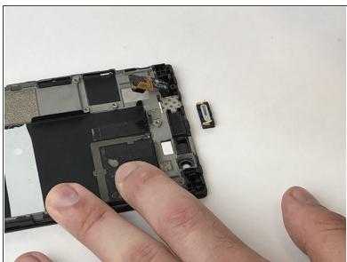
Using the plastic opening tool, remove the speaker.
