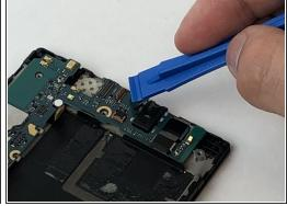
• Disconnect the camera from the motherboard with a plastic opening tool.
