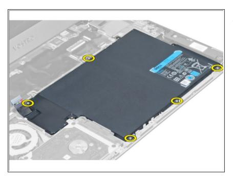
Remove the screws that secure the battery to the system board.
