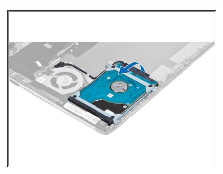
Lift the hard drive to disconnect the hard-drive cable
