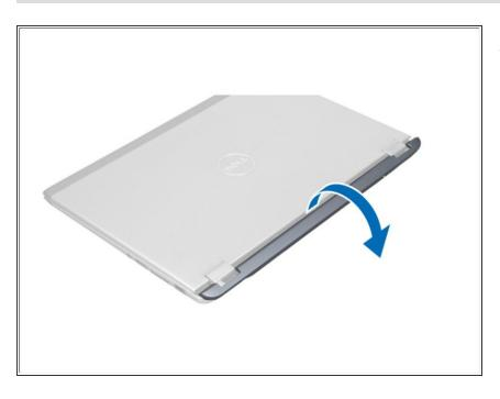
Remove the display-hinge cover from the computer.
