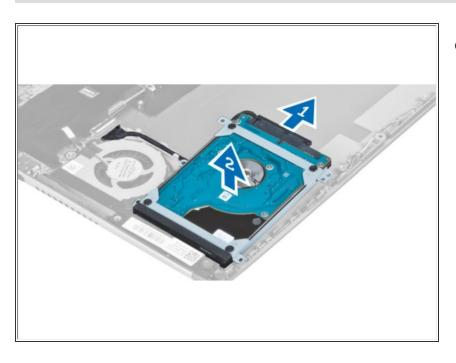
Disconnect the hard-drive cable from the hard drive and remove the hard drive from the computer
