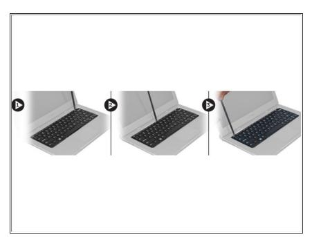
• Starting on the right side of the system, use a plastic scribe to pry up the keyboard from the computer.
