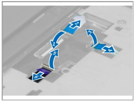
Disconnect the quick launch board cable, the finger print reader cable, and the palmrest cable from the system board.
