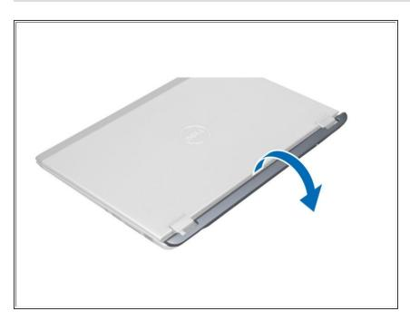
• Remove the display-hinge cover from the computer.
