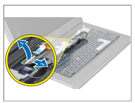
• Lift the clip to release the keyboard cable and disconnect it from the computer.
