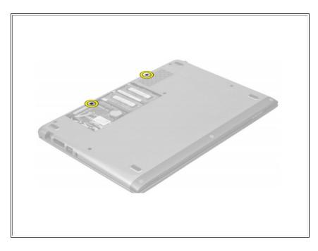
• Remove the screws that secure the display-hinge cover to the computer
