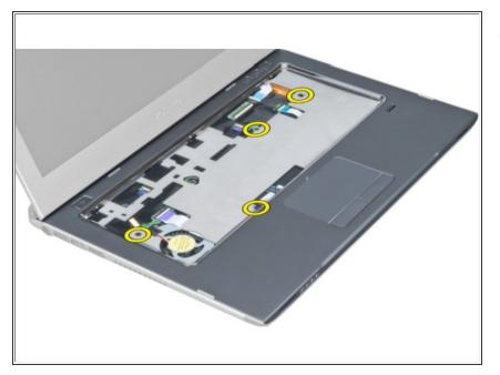
Remove the screws that secure the palmrest to the front of the computer.
