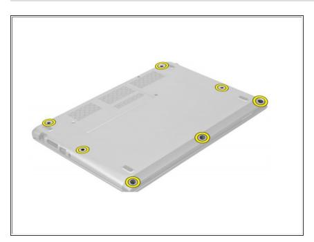
• Remove the screws that secure the palm-rest to the computer.
