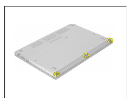
• Using a plastic scribe pry out the rubber pads that cover the front screws on the base cover.
