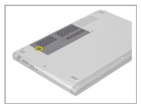
• Remove the screw that secures the access panel to the computer.
