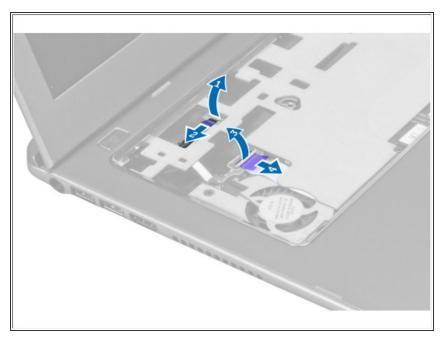
• Disconnect the power LED cable and the LED board cable from the system board.
