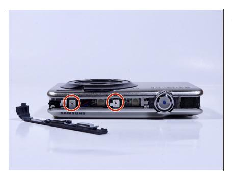
Remove screws beneath the top panel indicated by red circles with a #00 Phillips driver.
