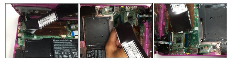
• Lift the pins holding the keyboard cable in place and slide the cable out to disconnect the keyboard.
