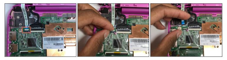
• Unplug the power jet, by lifting the pin and sliding the cable out.
