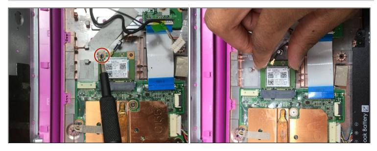
• Remove the screw securing the WiFi card in place using the JIS 4mm JO bit. Slide the card out of its socket.
