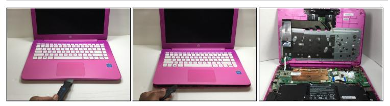
• Flip the laptop back up so that the HP logo is facing up. Open the laptop so that the screen and keyboard are showing. Insert the jimmy tool to remove the casing around the keyboard/touchpad area. Move the jimmy around the perimeter to loosen the casing. Remove the casing to reveal the guts of the laptop.
