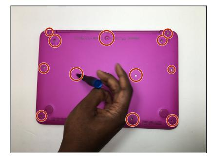
Remove the screws on the bottom of the laptop, as well as the screws under the rubber bumpers, using a JIS 4mm JO screwdriver. There should be 13 screws total.
