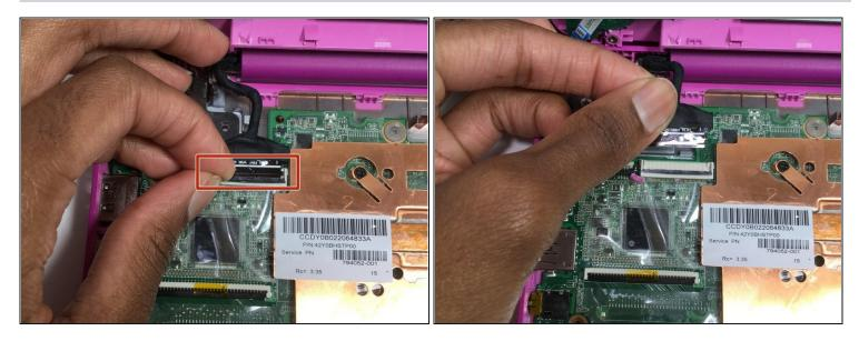
• Lift the pin up and unplug the video cable pin to disconnect it from the LCD.
