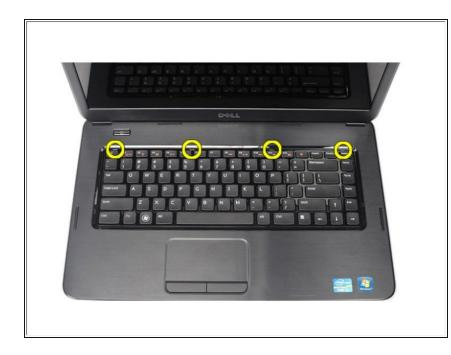
• Pry up to release the tabs securing the keyboard to the computer.
