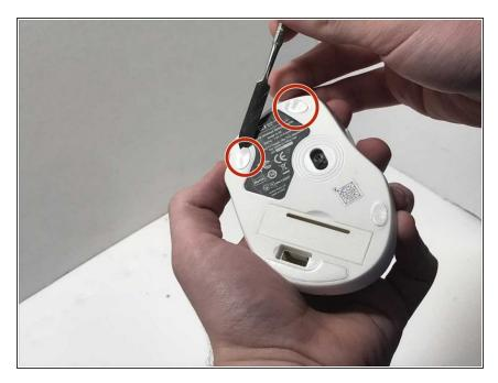
Remove the battery cover, and batteries from the compartment.
