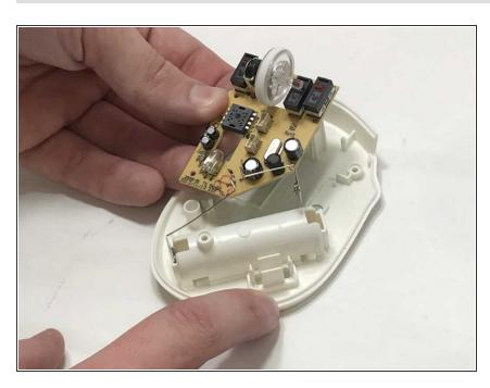
Remove the circuit board from the plastic base of the mouse.
