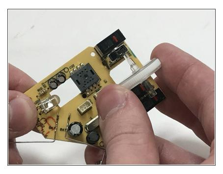
Move the wheel away from the rotary encoder, and lift it to remove it.
