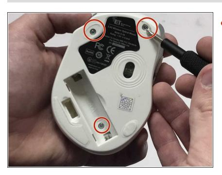
Use a Phillips #000 screwdriver to remove the 3 screws.
