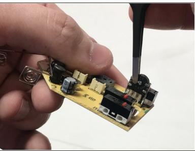
Use tweezers to squeeze the rotary encoder. Do this in multiple spots.
